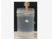
Silica-silica composite depot after injection into gelatin gel
